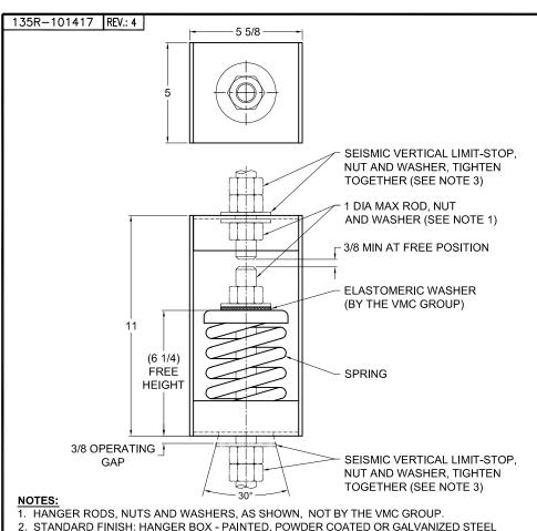
3. SEISMIC VERTICAL LIMIT-STOP REQUIRED FOR SEISMIC APPLICATIONS. NOT BY THE VMC GROUP. INSTALL WASHER .16 THK. MIN. X 3 O.D. MIN. WITH REQUIRED INSIDE DIAMETER TO ACCOMMODATE ROD SIZE IN USE. THIS CAN BE ACCOMPLISHED BY USING A SINGLE WASHER OR BY STACKING NOT MORE
